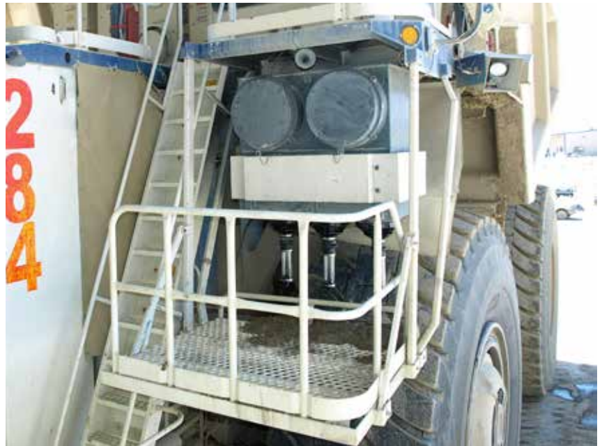
Dust Dumpa kits installed on a Donaldson SSG29 with rain shields. Notice the piles of dust gathered on the platform during vehicle operation.
