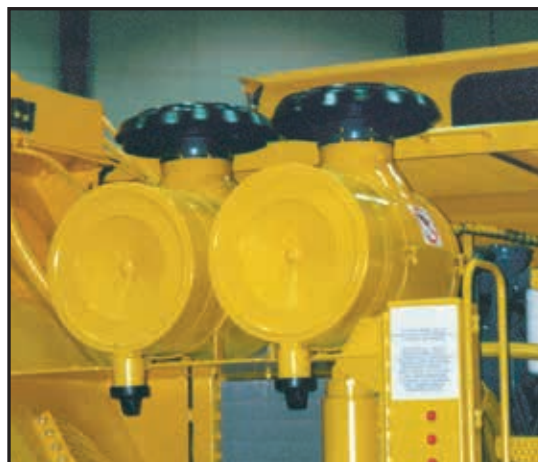
FVG air cleaners are used in tandem on this underground mining equipment to double the airflow throughput to the engine.
