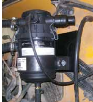
FIGURE 4 SPIRACLE SYSTEM ON A SCHOOL BUS
